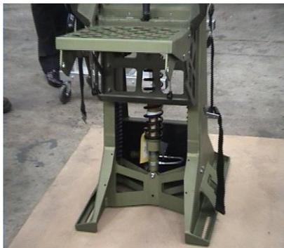
**Figure 3. Sub-Assembly of Suspended Seat With Shock Isolator**
